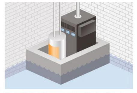
Because of hydrostatic pressure, component floodproofing barriers should designed to a maximum of 3 ft.
